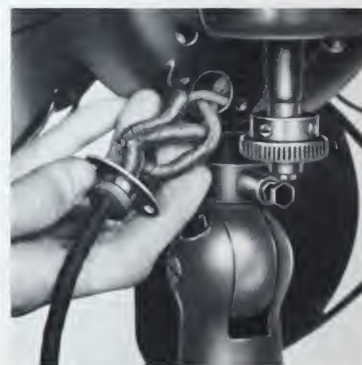
Oscillating Cord Easily Replaced
